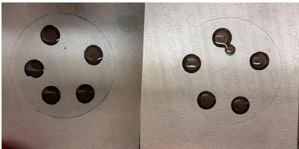
Figure 1. Chlorite after 1 hour. Chlorite reacts with the coating.
