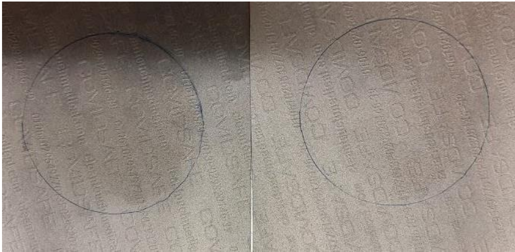
Figure 4. Ethanol 70 t-% after 1 hour. No visible changes. The liquid appears to have evaporated from the surface.
