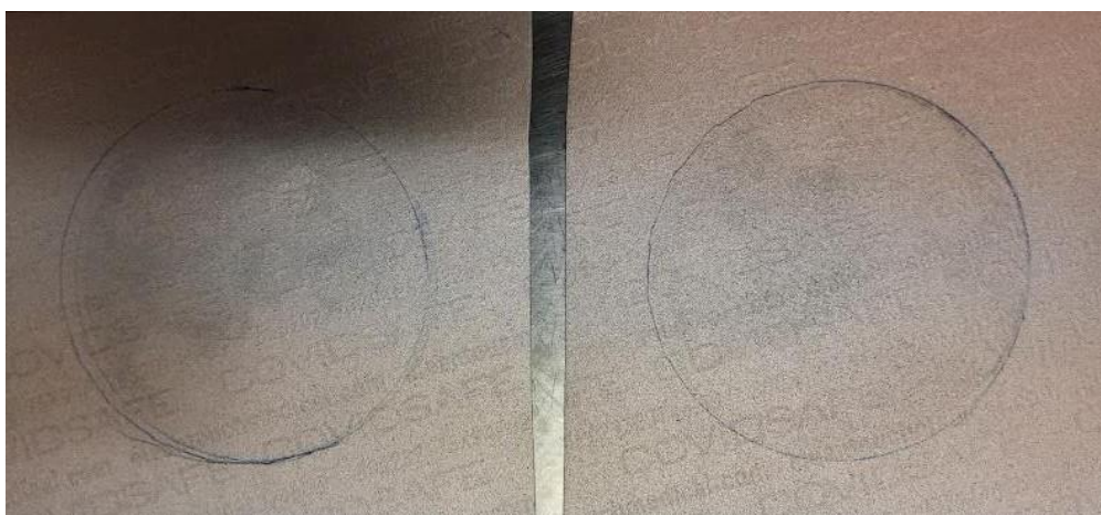
Figure 3. Membrane with additive, ethanol 70 t-% after 1 hour. No visible changes. The liquid appears to have evaporated from the surface.
