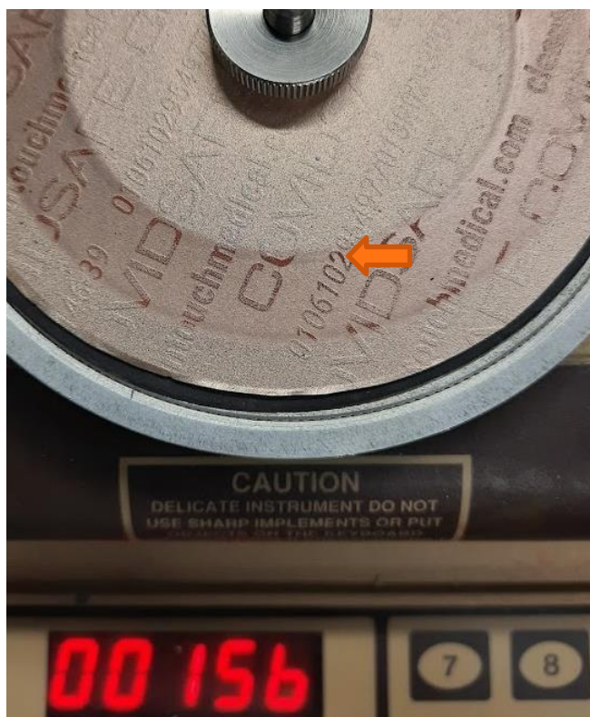
Figure 3. Test piece 3. Puncture-abrasion visible at 156 rpm.
