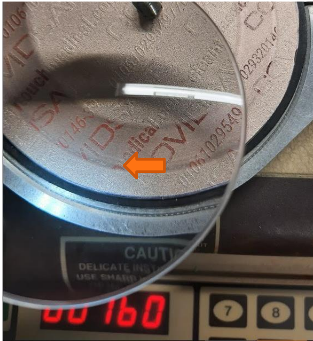
Figure 1. Test piece 1. Puncture-abrasion visible at 160 rpm.
