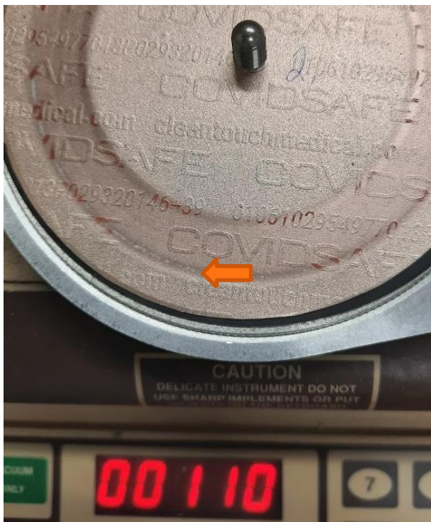
Figure 2. Test piece 2. Puncture-abrasion visible at 110 rpm.
